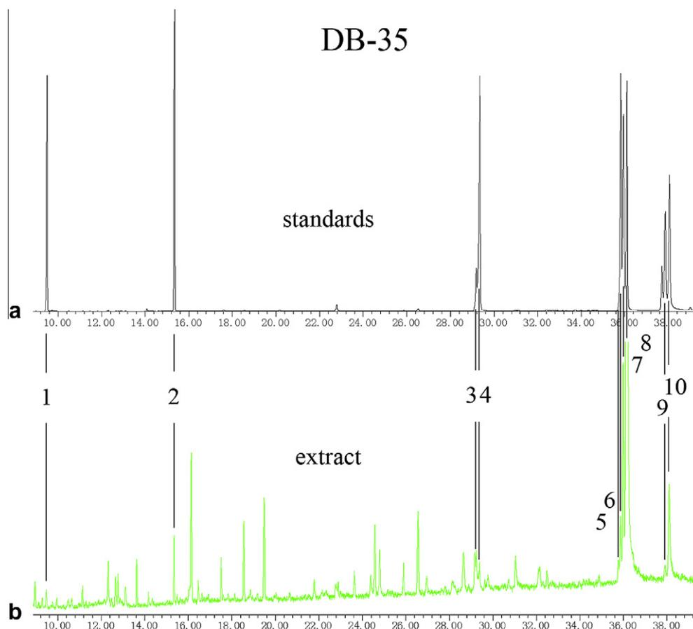
**Fig. 3.** Identified gland extracts of calling females by GC–MS equipped with capillary column DB-35. (a) Total ion current chromatogram from synthetic standards. (b) Total ion current chromatogram from pheromone gland extracts of female calling *Helicoverpa armigera*. Peaks from 1 to 10 are heptanal, nonanal, tetradecanal, (Z)-9-tetradecenal, (Z)-7-hexadecenal, (Z)-9-hexadecenal, hexadecanal, (Z)-11-hexadecenal, 1-hexadecanol, and (Z)-11-hexadecanol.
